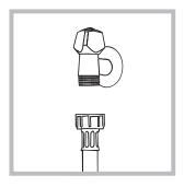
1. Connect the supply pipe by screwing it to a cold water tab using a <sup>3</sup>/<sub>4</sub> gas threaded connection (see figure).
